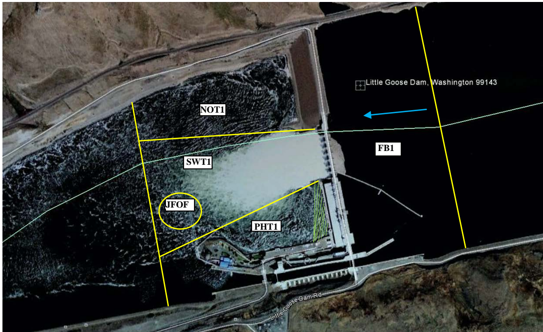
Figure 28. Zone map used at Little Goose Dam in 2012. Yellow lines demarcate zones, green lines represent the deterrent lines downstream of the powerhouse (not exact number), and the blue arrow indicates flow direction.
